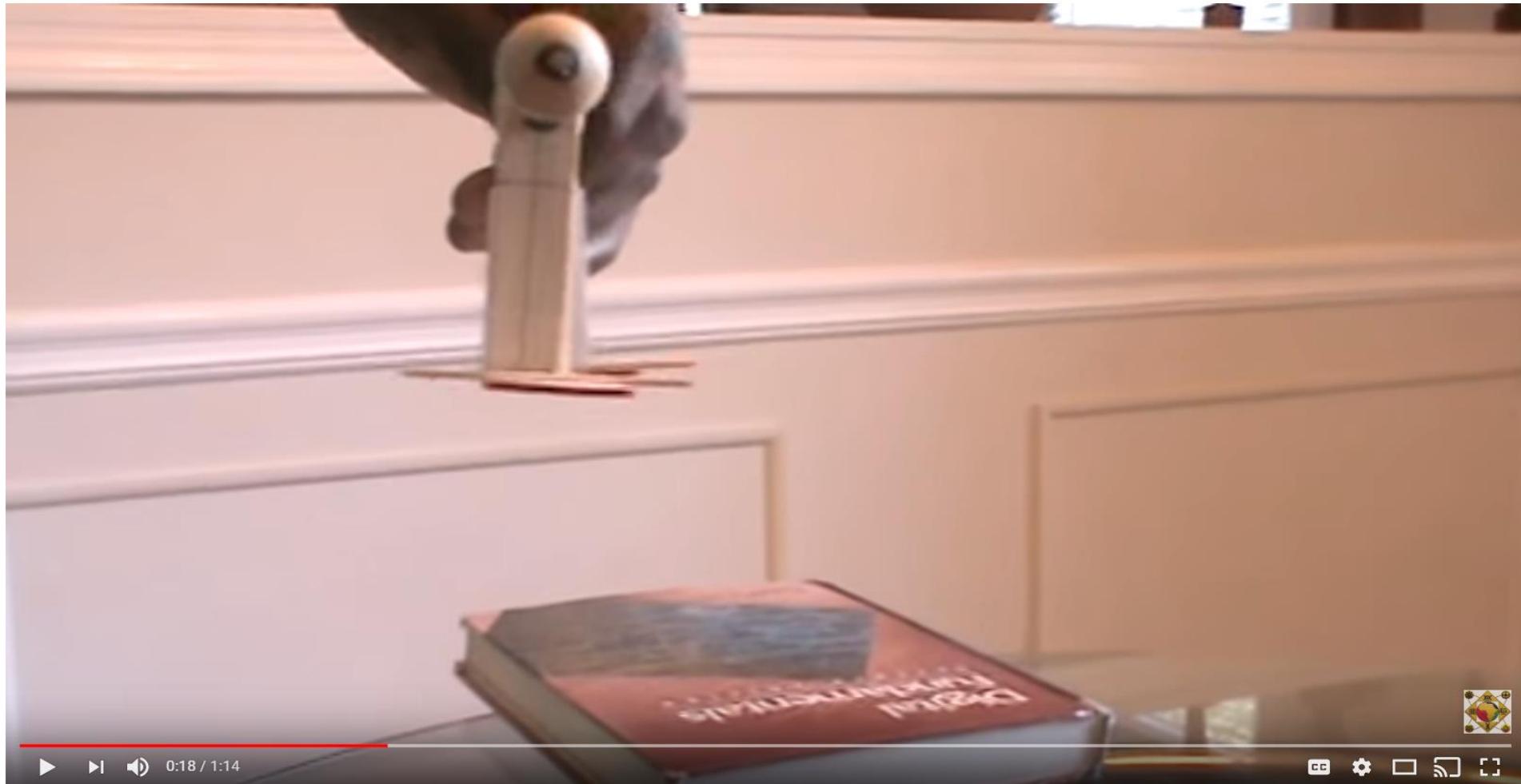
Passive Dynamic Robotic Walker trial_2 - 7cm popsicle stick legs
